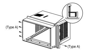
Frame When the frame guides are set, the arrows should be pointing toward the back end of the unit.
